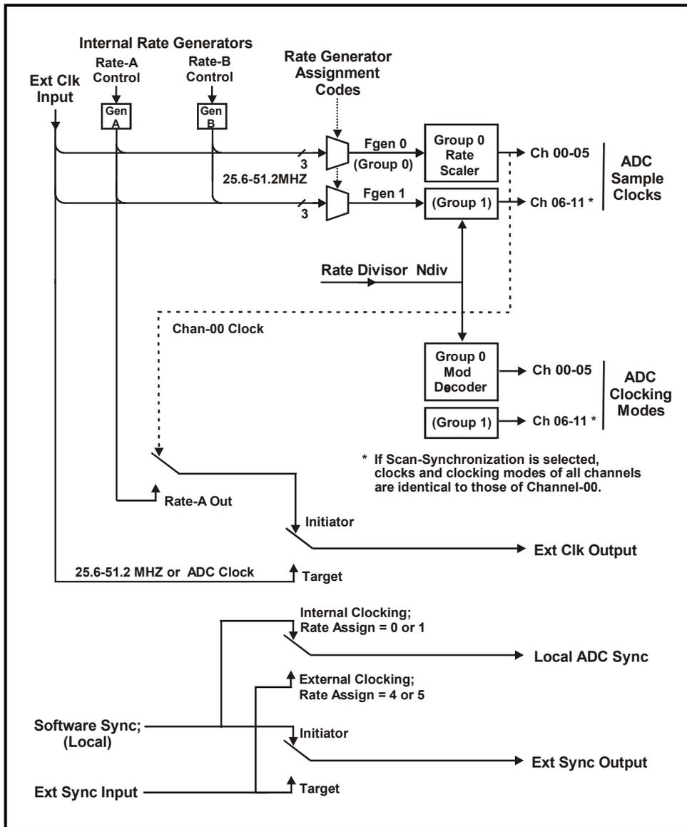
Figure 3.6.1.1. ADC Clock and Sync Organization, 12 Channels
