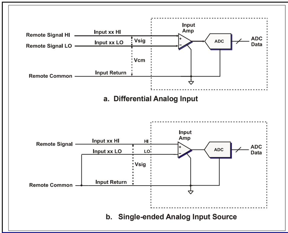
**Figure 2.3.1. Input Configurations**
