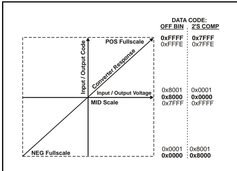
Figure 3.6-1. Analog Data Coding Formats; 16 Bit Data
