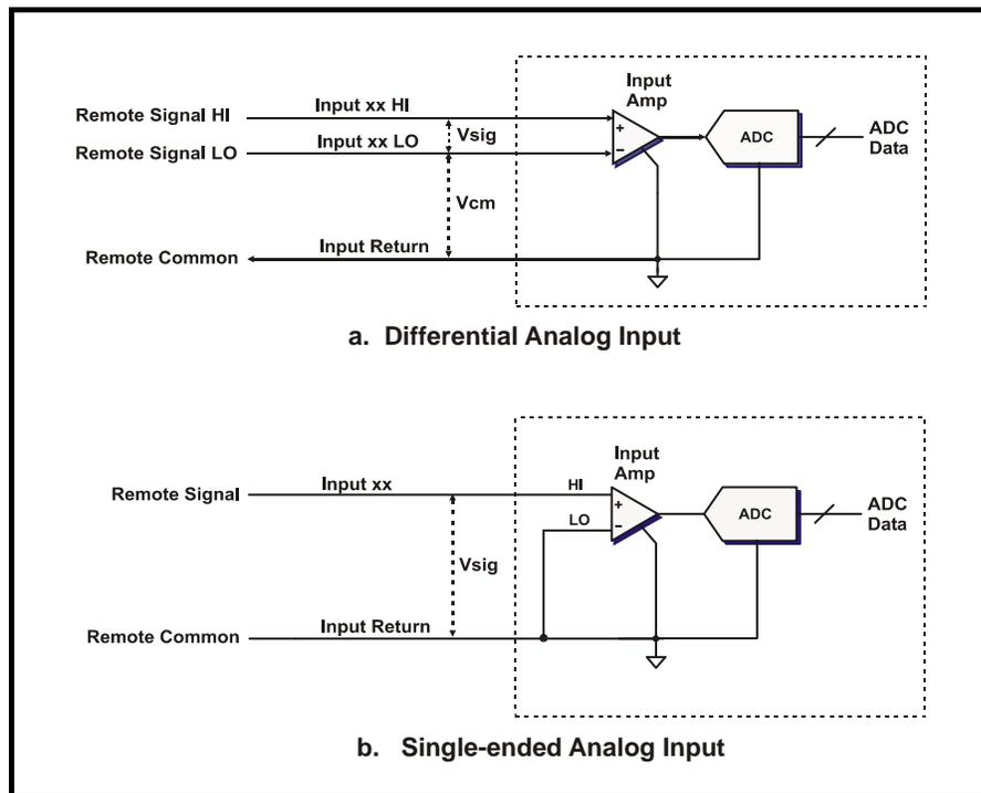
Figure 2.3-1. Analog Input Configurations
