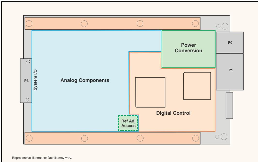
**Figure 2.5-1. Reference Adjustment Access**
