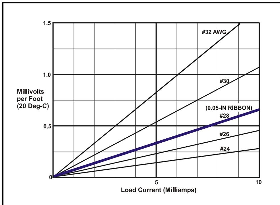
Figure 2.3-3. Line Loss versus Load Current
