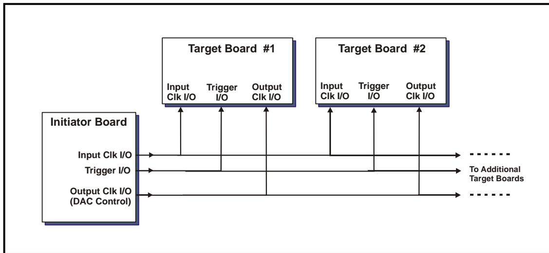
**Figure 2.3-4. Multiboard Synchronization**
