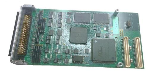
The PMC-HPDI32B-COS is a 32-bit parallel Change of State Detection board featuring high speed RS485 interface transceivers. The Change of State detection is can be customized to ignore specific bits and to provide an interrupt after a specified number of change of state events have occurred. The board will also function as a simple Logic Analyzer with a configurable trigger value and mask. The sample rate for both Change of State and Logic Analyzer is programmable from 20MHz down to 300Hz.
